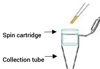
Figure 1. Spin Cartridge/Collecting Tube Assembly
