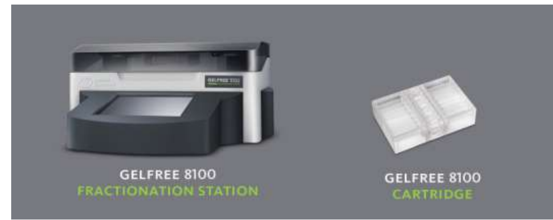
Figure 1. The Gelfree 8100 instrument (left) is an eight channel electrophoretic controller that supplies voltage independently to each of the eight channels in the pre-cast cartridge (right). A touch screen display located on the front of the instrument allows the user to program the voltage to apply to each channel, as well as the fraction collection intervals. To use the system, the user programs the sequence (or chooses from a pre-programmed sequence) for each of the eight electrophoretic channels and starts the experiment. The device automatically pauses the experiment whenever the time interval has expired, allowing the user to extract the molecular weight fraction of interest. Measurement information for the eight channels is displayed to the user in tabular and graphical format during the course of an experiment.
